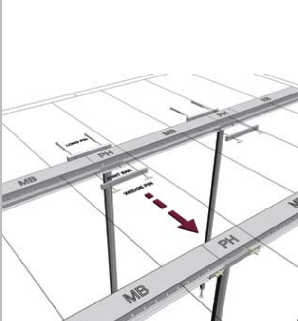
1 Dismantle long pins & joint bars from prop heads
