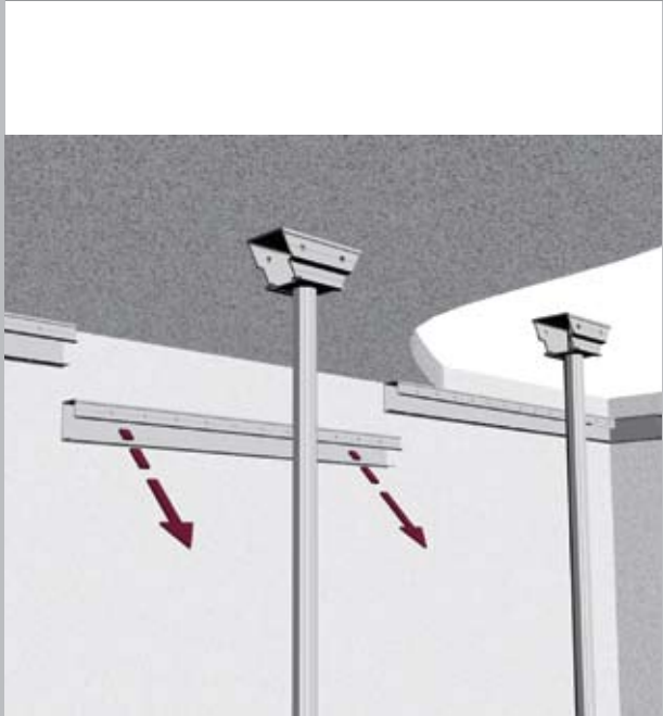
4 Dismantle outer middle & end beams
